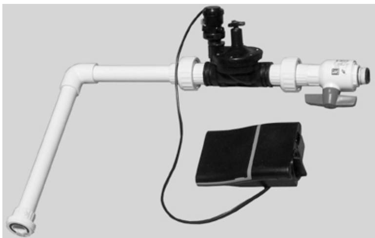
Internal Wash Timer Assembly
